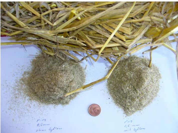
With the Cyclone separator and a 0,25 mm sieve cassette, 1 kg dry straw was put through in 10 minutes. In order to understand this amount better, refer back to the volume of 1kg uncomminuted.
