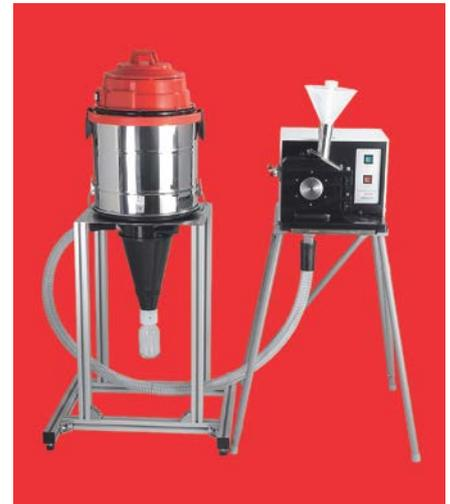
Straw was comminuted with a Universal Cutting Mill PULVERISETTE 19, equipped with a 0,5 mm sieve cassette. During the first test, the sample was processed without the Cyclone separator, for the second test the Cyclone separator was used. When comparing both finenesses, the sample processed with the Cyclone separator contains slightly longer shares. In the air current generated by the Cyclone separator, longer parts are rather aligned and pushed through the sieve.
